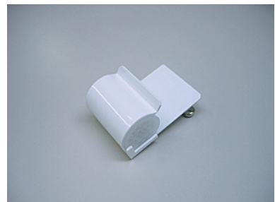
Average gas concentration estimated through simplified measurement using a passive sampler.
